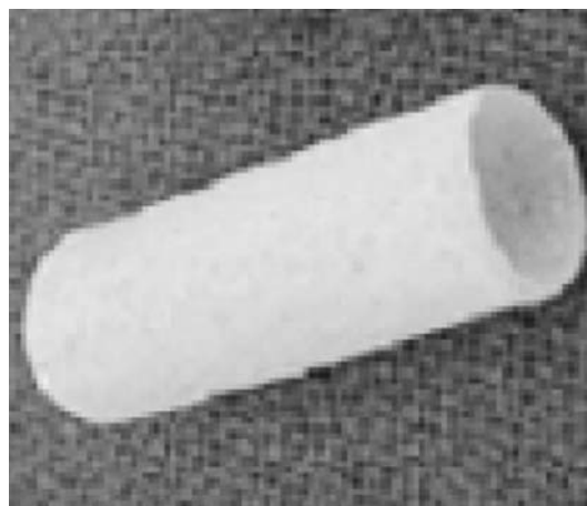
Fig. 1 The scaffold Length \times Thickness \times Diameter \approx 20 mm(L) \times 0.2 mm(T) \times 4 mm(D)
